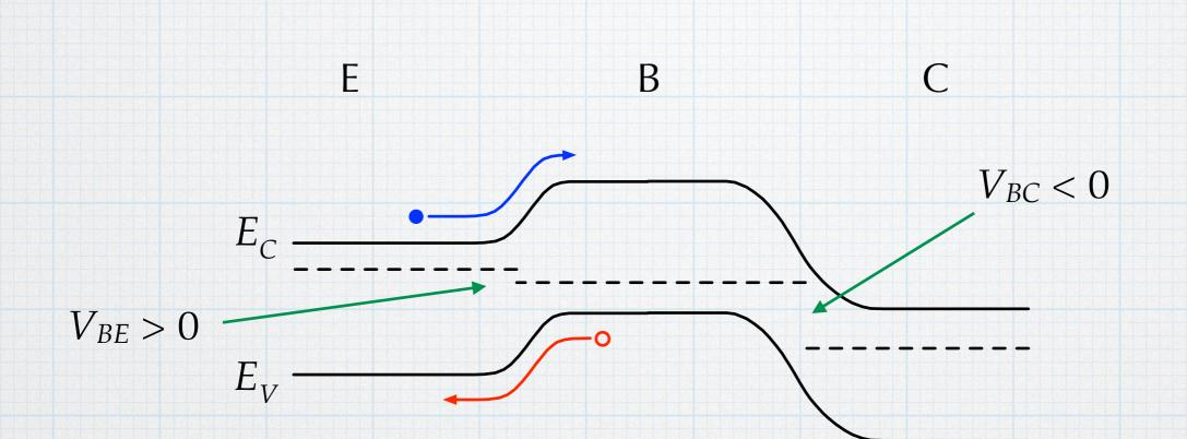
Electrons and holes will be injected across the base-emitter junction. No injection across the base-collector junction.
