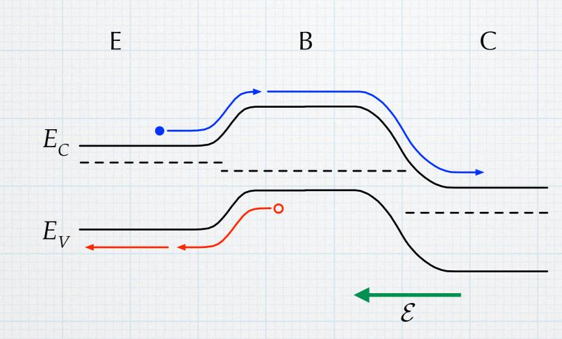
The electrons will diffuse across the base region. When they get to the high electric field at the B-C, they will be swept across and into the collector. They end up as collector current!
