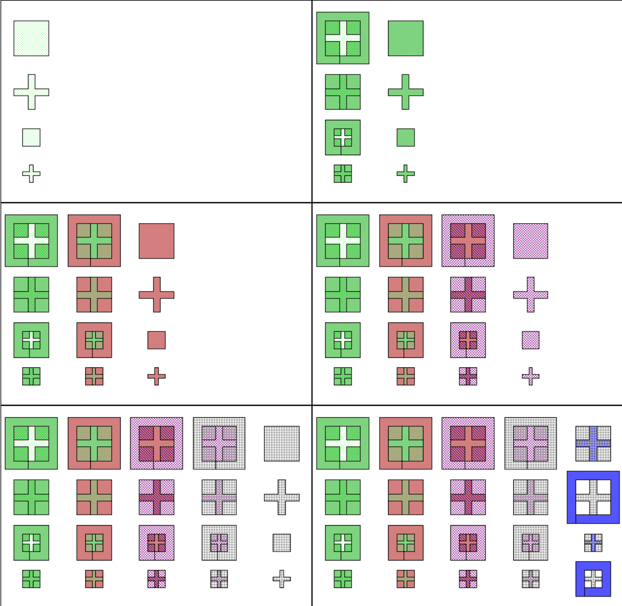
Figure 4: Alignment Marks Layer by Layer
