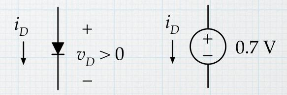
Note that the diode is NOT a voltage source. It is a passive device and does not provide power to the circuit. But it does behave as if it were a voltage source or battery that is absorbing power.
