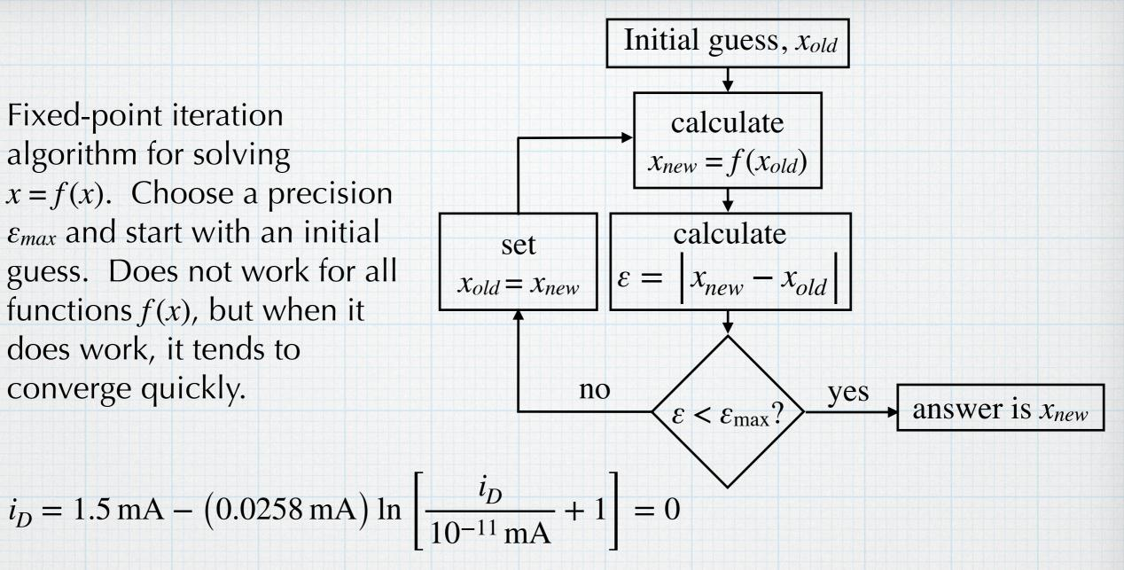
Applying the method to our diode equation, with an initial guess of 1.00 mA, gives the sequence shown. Within four iterations, the calculation has converged to 5 significant digits.
