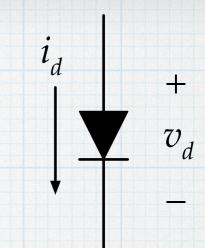
where  $i_D$  is the diode current and  $v_D$  voltage across the diode. As stated earlier, the relationship is extremely non-linear, and it will cause us a some grief when analyzing diodes. But the non-linear behavior offers opportunities for new applications.
