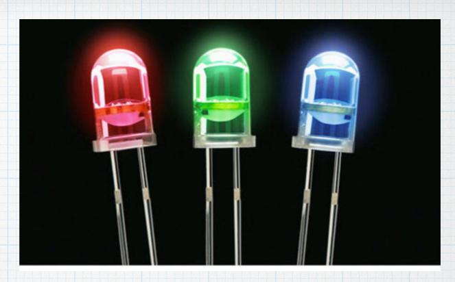
LEDs – various materials (not silicon). Different material = different colors.
