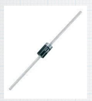
rectifying diode (switching or small-signal)
