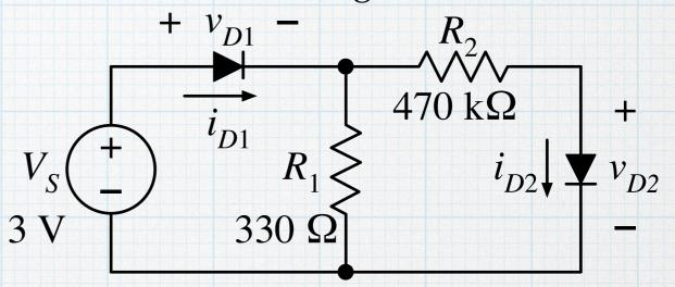
Try node voltage (ground at the bottom, two node voltages  $v_{R1}$  and  $v_{D2}$ ):
