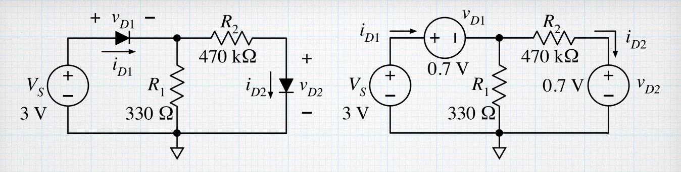
Having replaced the diodes with fixed voltages, the circuit analysis is nearly trivial.
