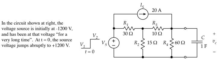
Find the effective *RC* constant for the circuit (Note unusually large value of the capacitor.) Determine the expression for the capacitor voltage as a function of time (with the correct numbers, not just variables). Determine the time at which the capacitor voltage crosses +500 V.
