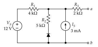
(Note: We know that the Thevenin theorem does not work when non-linear devices, like diodes, are present. However, we are modeling the behavior of the diodes with *linear* approximations – either a 0.7-V diode drop or an open circuit – so the Thevenin equivalent will be OK, within the limits of the approximation.)
