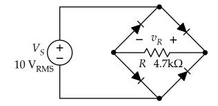
(a) What will be the peak value of the rectified voltage waveform?
