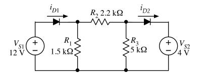
Then repeat the calculation with  $V_{S2} = 12$  V.
