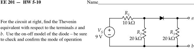
(Note: We know that the Thevenin theorem does not work when non-linear devices, like diodes, are present. However, we are modeling the behavior of the diodes with *linear* approximations – either a 0.7-V diode drop or an open circuit - so the Thevenin equivalent will be OK, within the limits of the approximation.)
