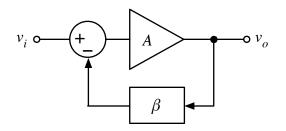
a. If the open-loop gain has a nominal value of 100 with a variance of  $\pm 50\%$  and the feedback is perfect with a value of 0.0667, calculate the nominal, high, and low values of the closed-loop gain.
