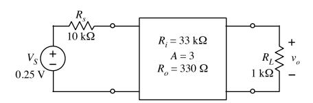
a. Calculate the voltage gain,  $v_o/V_S$  for the single stage amp:  $A_{T1} =$
