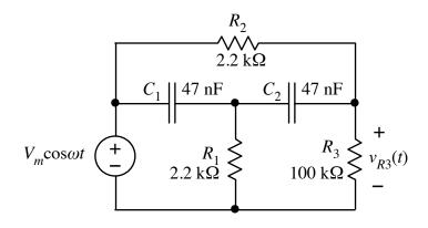
Note that there will be a transient at the start of the simulation. Determine the amplitude and phase shift from from the later periods of the plot, after the transient has disappeared.
