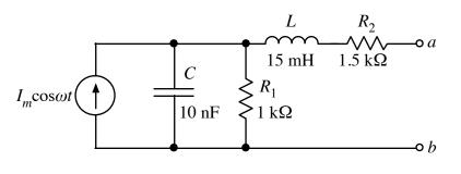
The amplitude of the source is  $I_m = 10$  mA, and the angular frequency is  $\omega = 10^5$  rad/s.
