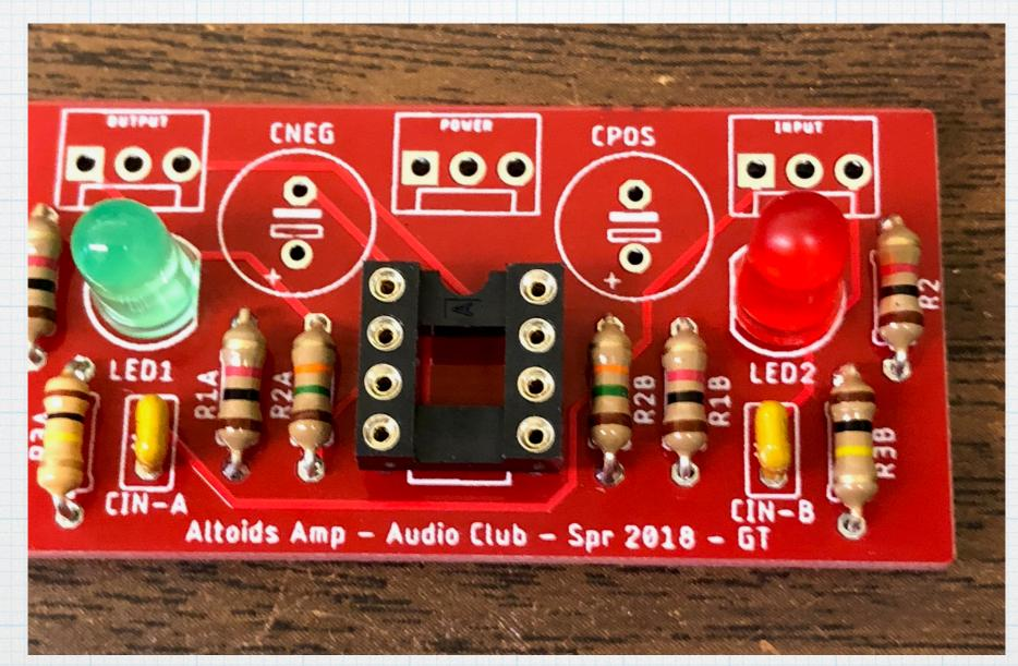
Note: The LEDs are not absolutely necessary. If you want, you can leave out the diodes and resistors entirely without affecting the operation of the amplifiers. You can also use different colors, if you want.
