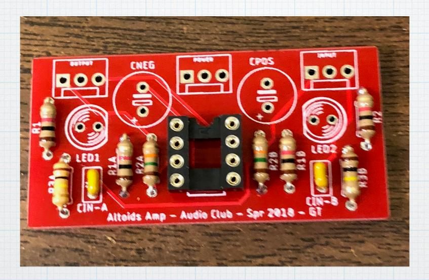
Note: The LEDs are not absolutely necessary. If you want, you can leave out the diodes and resistors entirely without affecting the operation of the amplifiers. You can also use different colors, if you want.
