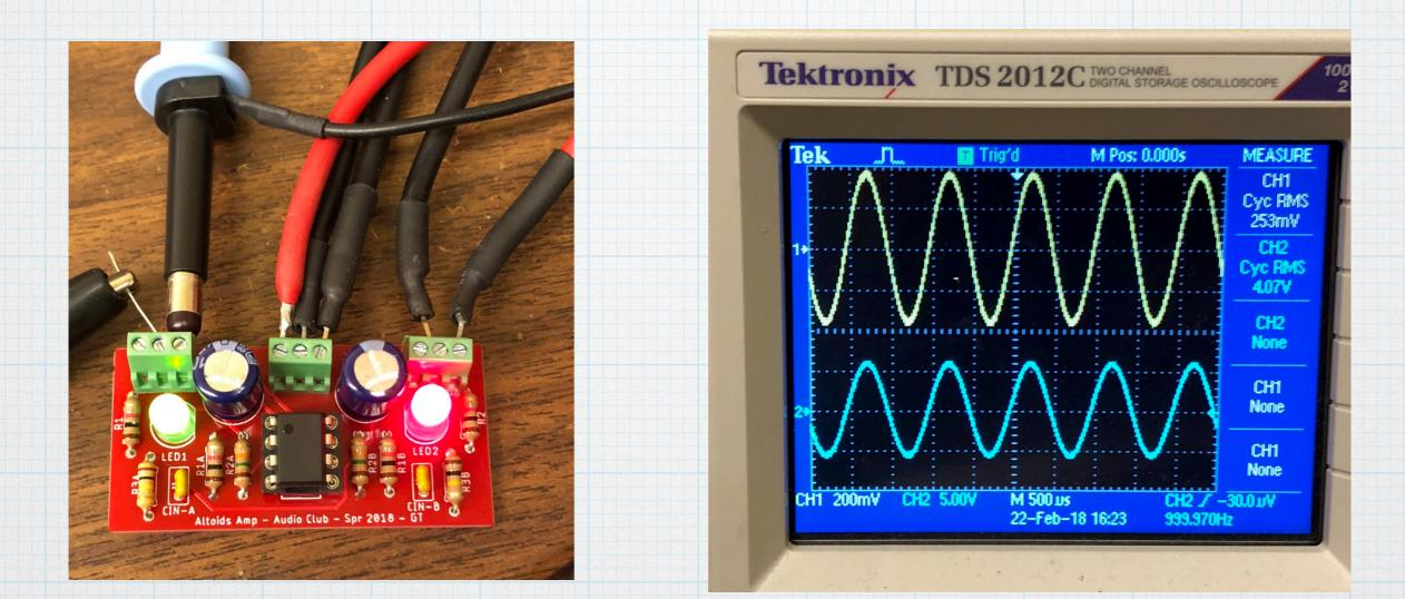
Both channels give similar results - clean output with gain of 4.07 V / 0.253 V = 16.1 — as expected.
