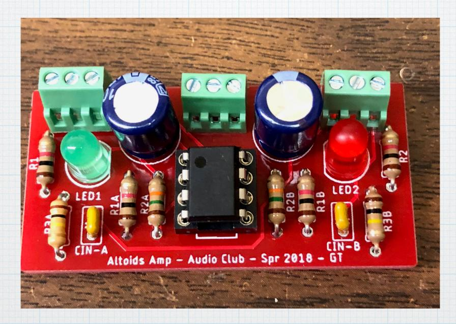
It is probably necessary to bend in the pins a bit in order to get the chip to insert into the socket easily.
