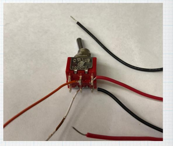
Cut two pieces of lead wire — about 2 inches long — and solder these to the center connections of the switch. Keep track of which is which. Here, the orange wire is on the same switch as the red battery lead — this is the positive power supply lead. The brown/white wire goes with the black battery lead, and this will be the negative supply lead. (Your colors may vary, depending on where you get your lead wire.)
