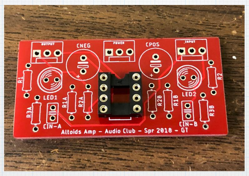
Note: A socket is not absolutely necessary. You can solder the op-amp chip directly to the board. But if you do that, it becomes very difficult to remove the chip if it is burned out or you would like to try a different amplifier.
