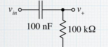
The input *RC* combination serves as a high-pass filter ( $f_c = 16$  Hz). More importantly, the series capacitor provides decoupling to prevent DC voltages from accidentally damaging our music source.
