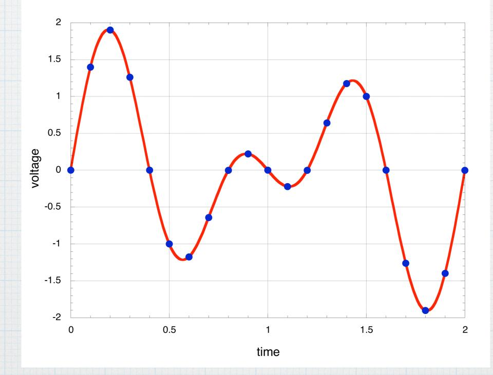
Measure the voltage every  $\Delta t$ . In this case,  $\Delta t = 0.1$  s. (Sampling rate of 10 samples/sec.) All voltages are still possible, but we are looking only at specific discrete points in time.
