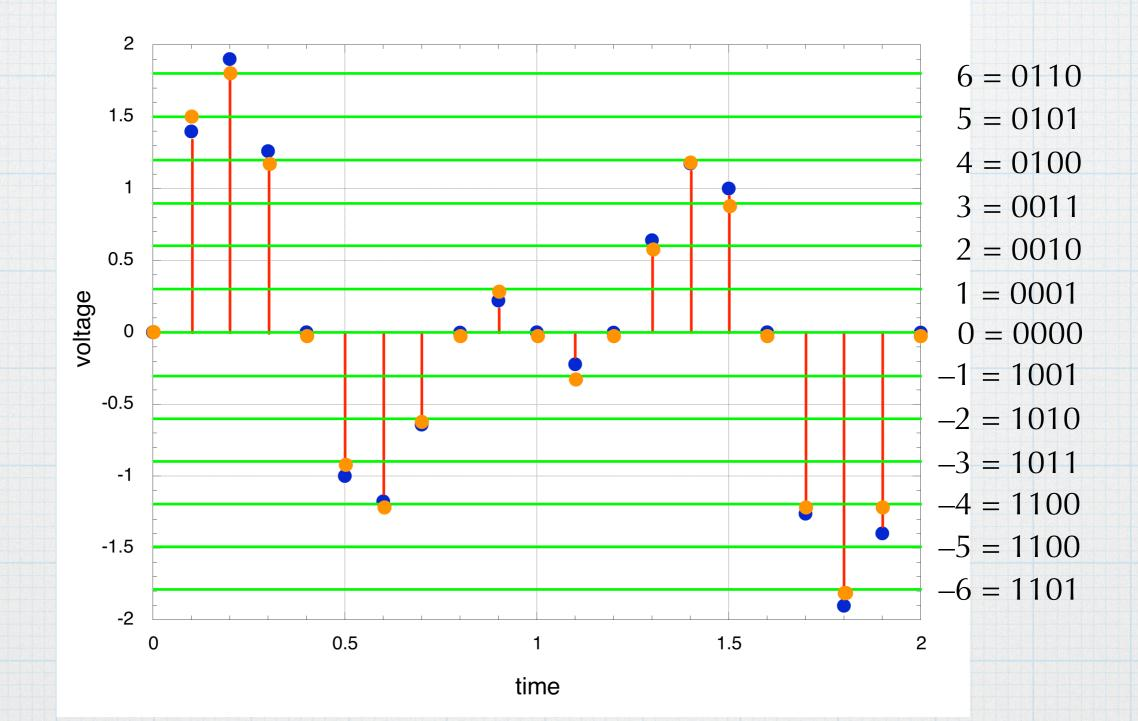
Slice the voltage range into equal-sized chunks. Represent each chunk with a binary number. In this case, we used 4-bit signed binary numbers (–7 to +7), with each chunk 0.3 V wide. There may be some *quantization error*.
